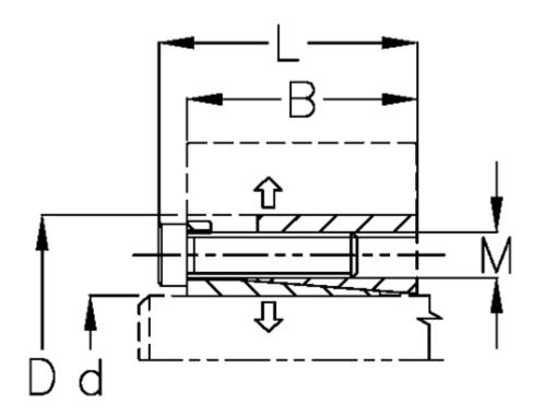
$\begin{array}{lll} \text{B mm} & = 72.0 \\ \text{d H8 mm} & = 260 \\ \text{D mm} & = 325 \\ \text{Fit tolerance} & = \text{Aksel h8, Nav H8} \\ \text{F kN torque} & = 1017 \\ \text{L mm} & = 88 \\ \text{M mm} & = \text{M16} \\ \text{P N/mm2 surface pressure on shaft/hub} = 174 \\ \end{array}$
